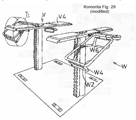
Figure 29 of Komorita depicts tire hanger W extending from the side of lift V.<sup>10</sup> Tire hanger W consists of a "tire receiving main swing arm W2
