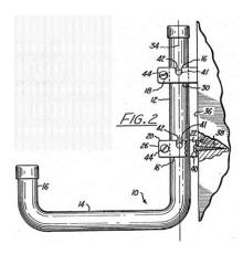
As described by Conrad, the utility hook includes a vertical section and a horizontal section. *Id.* at 2:6–8. The vertical section is supported by "bracket means [] which extend into the wall of the support structure, on which the apparatus is mounted." *Id.* at 2:28–30. Conrad further teaches that "the hooked end of the horizontal section may be provided without a full
