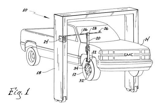
According to Heidle, the S-hook fastener is "operatively arranged to fasten to the wheel." *Id.* at 1:50–53; *see also id.* at 3:1–2 ("Fastener 22 is secured to wheel 12 by removing any slack in strap 20."). Once the lug nuts of the wheel are removed, "wheel 12 is pivoted away from vehicle 14 and suspended by hoist 10." *Id.* at 3:17–22. As a result, "[t]he mechanic then avoids having to drop *or lift the wheel.*" *Id.* at 2:27–30 (emphasis added).
