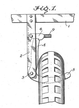
As described by Marion, the hook member supports the tire "in display position" so that it "may be removed and replaced with the least possible trouble." *Id.* at 1:9–16. Lifting the tire upwardly disengages a "latch" on the hook member, permitting the hook member "to swing downwardly . . . and consequently allowing the tire to be drawn downwardly
